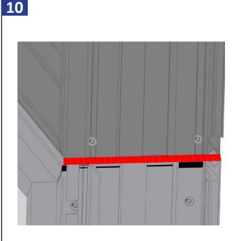
Cover the joint at the head and sill with sealant and tool flat as shown above.
