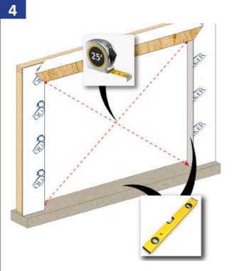
Check that the opening is square. The diagonal measurements need to be within 1/8" of each other. Verify the rough opening is plumb and level.
