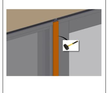
Take the interior mull cover (Die #: M25408) and snap it over the interior mull to cover fasteners. FOR WOOD USE MULL COVER (BRS-9478)
