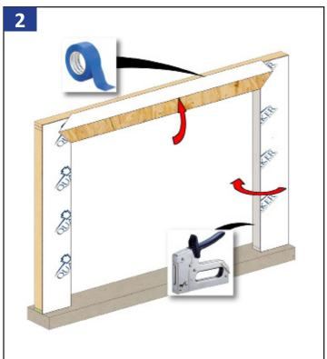
Fold the house wrap around the jambs to the interior and staple it to the interior framing. Fold the house wrap flap up and temporarily tape it in place.
