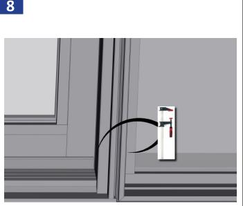
Place the units together making sure they are flush and level. Apply a hand clamp to keep the units together.
