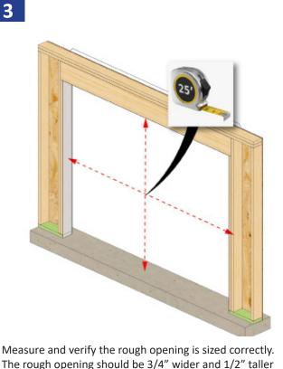
Measure and verify the rough opening is sized correctly. The rough opening should be 3/4'' wider and 1/2'' taller than the unit. Allow additional space for flashing thickness, installation clips, joining components, and their fasteners.
