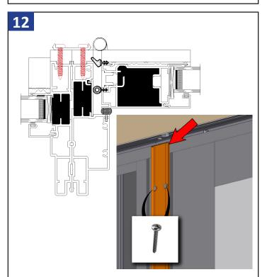
Place the interior mull (Die #: M25407) on to the face of the door. Drill a hole 11/64" hole through the wood and the aluminum leg. Drill a hole in each die line, 3" from each end and then 16" on center, as shown above. Then install fasteners #10, 1.25", (Part #: 0171859).
