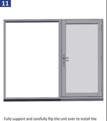
Fully support and carefully flip the unit over to install the interior mull.
