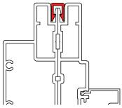
Cut the C-mull keys to the length on the exterior side of the unit. Install the mull with a mallets by tapping the mull key into the tracks. This will lock them together as shown above. You may need a block and hammer to drive the mull key in place.
